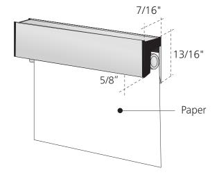
To insert the paper, simply slide it up in behind the aluminum rods.
