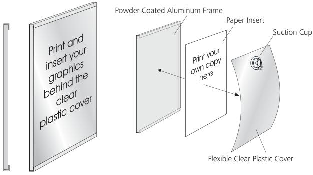
Side View 3/16" Approx. The cover is easily removed with the aid of a suction cup.
