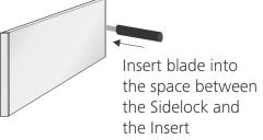
1. Simply slide the steel blade on the Custom Insert Removal Tool into the gap between the Frame and the Insert or Panel.
