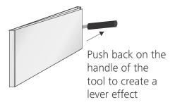
2. Once the blade is inserted, push down on the handle of the tool, creating a lever effect.
